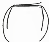
Example 6. Improper closure of the reed on the tip rail due to imbalance of ears.
