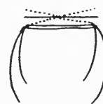
Example 4. Freely vibrating reed: Dotted lines indicate amplitude of ears' vibration.
