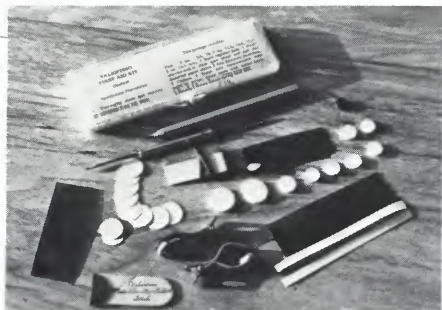
Photo No. 2. Here's what you get: a pencil, a combination tool where one end is a screwdriver and the other a spring hooker/pusher, a pad assortment, a hat pin, paper shims, a razor blade, two clamps, pre-cut self-adhering bumpers and tenon strips (to replace corks), and a Wha-Cha-Ma-Call-It Stick.
