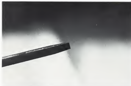
Photo No. 4. The screwdriver tip is well designed to seek and hold screw slots. It's on the light side so that damaging screw threads is difficult. A heavier screwdriver would be needed to remove rusted-in screws.
