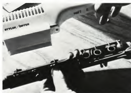
Photo No. 17. Here's another use for the Wha-Cha-Ma-Call-It Stick. The stick's black covered end is slid under the left hand F#-C# lever pressing down on the E-B lever while a hair dryer helps seat the E and F key pads for 30-45 seconds. A more conservative approach would use two clamps overnight, one clamp on each key cup.
