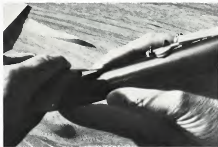
Photo No. 13. I'm pressing up like crazy on the front of the pad (the Stick is getting dented) while my right hand is holding the back of the key cup down. The pad has taken 20 minutes so far to install, and the frustration level is rising. (I'm ready to consider shimming.)
