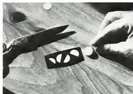
Photo No. 19. Not all pads will be level without shimming. Cut the paper shims to put more thickness where the pad leaks.
