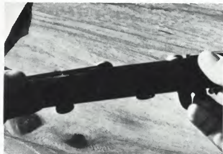
Photo No. 7. Shown here is the screwdriver cleaning the inside of the key cup. With the precision fit of Valentino pads, it's important that the sides of the cup are clean and that no old glue interferes with the level position of the new pad. Keep the key open when doing this. Hold the clarinet in a way that allows debris to fall away from the instrument, not into the bore. DO NOT TOUCH OR SCRATCH THE TONE HOLE SURFACE.
