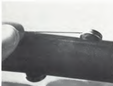
Photo No. 5. It's possible to install these pads without taking most keys off. Here the hat pin goes after the old pad. If the pad skin rips, dig out the felt and cardboard separately.
