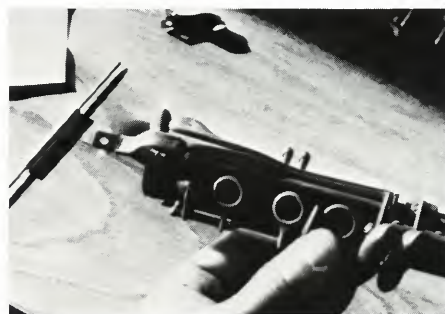
Photo No. 18. Another way to close the two large open keys, the clamp is holding the inside of the socket and the E-B lever. The ring key pad also needs clamping (or squeezing) to create a seat.
