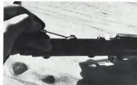
Photo No. 6. The screwdriver continues to work the old pad out. Be very careful not to touch or scratch the tone hole surface.
