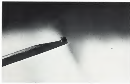
Photo No. 3. A close-up of the spring hook shows a first-class tool. The pusher works best on small needle springs.
