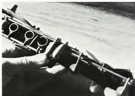
Photo No. 15. The pad seats well but is thicker than the old pad, creating a gap between the right hand F#-C# fingerpiece and the crowfoot. The left thumb is pressing the fingerpiece down while the right thumb holds the key cup closed.
