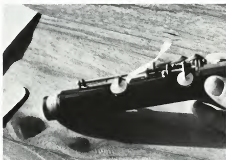
Photo No. 12. The pad's still gripping too lightly in back. I purposely chose a difficult pad to test the Valentino pad's ability to be shifted. Leaving the paper on the adhesive back helps, but it's still very hard to shift.
