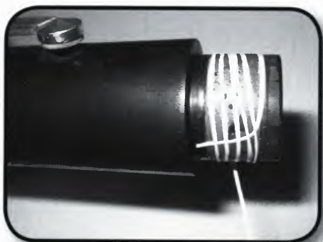
Example 16: Second Step: Wrapping Waxed Dental Floss around Cork.
